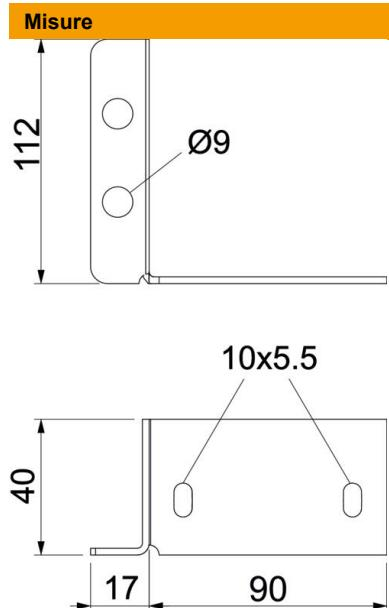
Front view dimensions: height 112mm, width 90mm, depth 40mm, side height 17mm, and a 10x5.5 slot.
