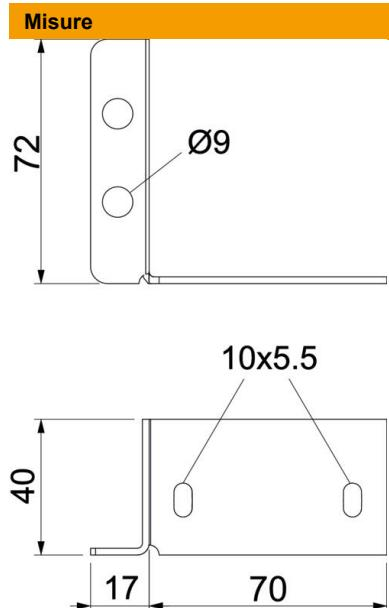
Front view dimensions: Height 72, Width 70, Depth 40. Side view dimensions: Height 72, Width 17.
